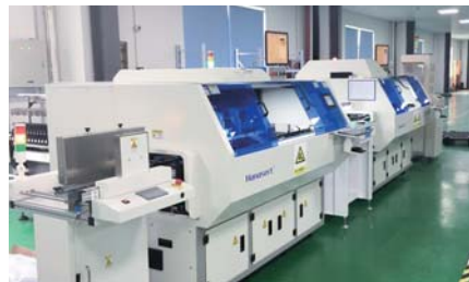
1. Universal Auto Insert Machine: Components automatically inserted to PCB, accurate and efficient.
