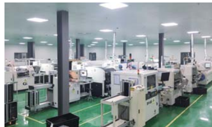
5. Automatic AOI visual inspection, which ensures every material properly used, material and PCB welding spot no lack of tin, insufficient solder and solder skips.
